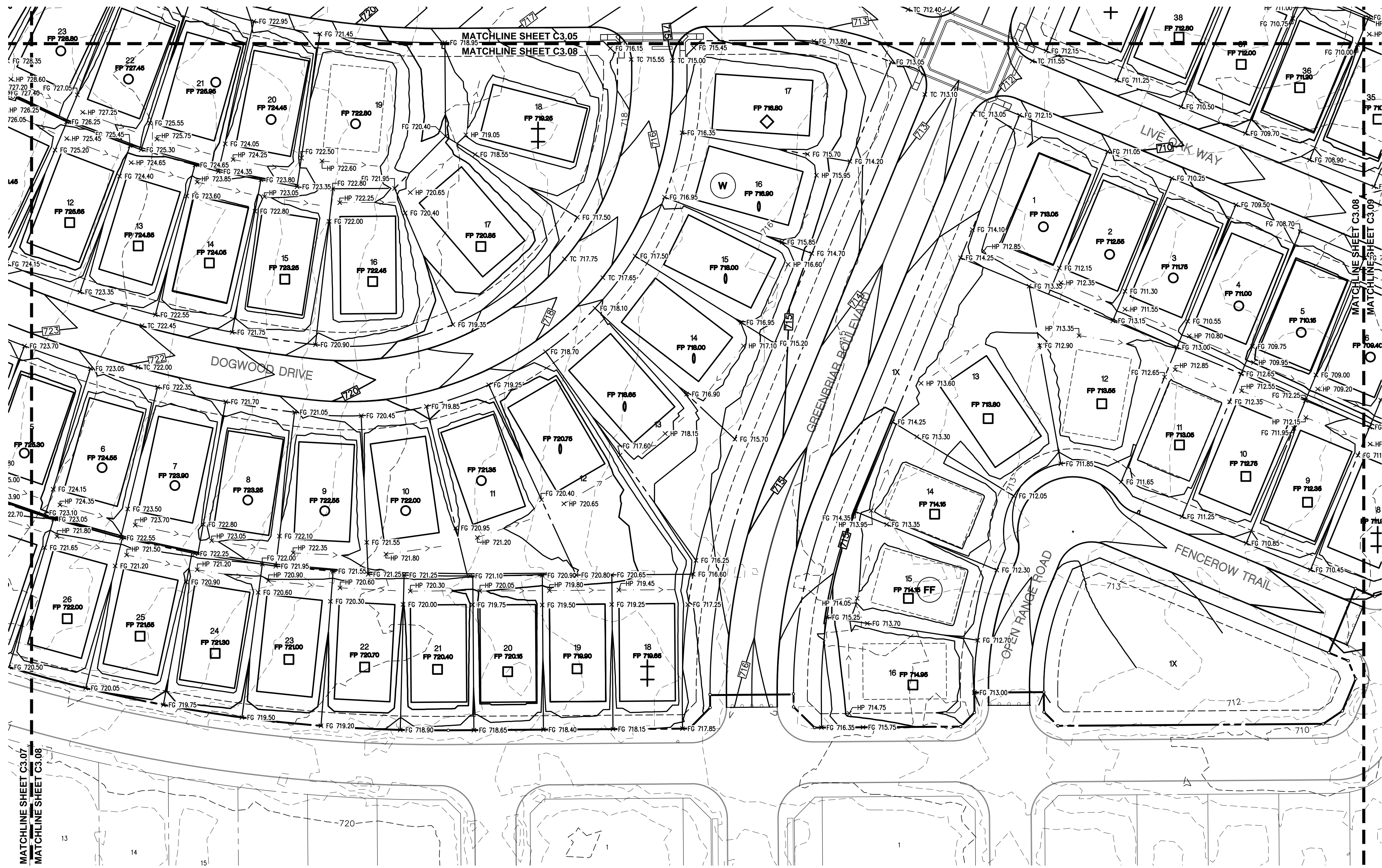
TYPICAL LOT GRADING KEY LOCATION OF HIGH POINT VARIES NOT TO SCALE
